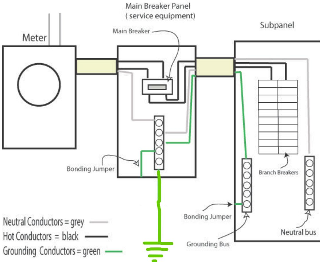
Do not GROUND the panel grounding electrode conductor to the meter base. You will BOND the meter base if using PVC from meter to the panel. The neutral is bonded at the first means of disconnect, such as a main breaker panel, disconnect or electrical panel. If a single ground rod is the only grounding electrode you must add a second ground rod a minimum of 6' away with an unbroken grounding conductor.
